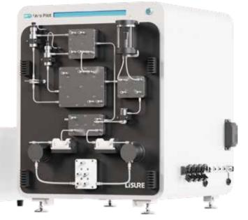
M++ is a cutting-edge innovation in downstream bioprocessing, a pilot-scale modular benchtop system that can run Chromatography, TFF, Depth Filtration (NFF), SSTFF, inline dilution (ID), and various process intensifications (PI) including 4C Continuous chromatography and many cycle-time-reducing integrated processes.
