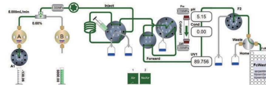
Despite the flow rate, all systems (36 ml/min, 100 ml/min, 300 ml/min) support injection through the sample loop. The illustrated system includes duo pumps, a fraction collector, a pH sensor, a conductivity sensor, a UV absorbance sensor and a temperature sensor. The sample can be manually injected into the sample loop, and the system will automatically switch the sample valve to Inject position at user defined time to fulfill the sample injection logic.
